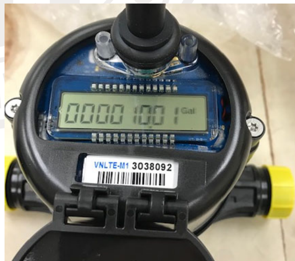
Figure 2. Top view of the meter with registration on a gallon unit of measure meter.
