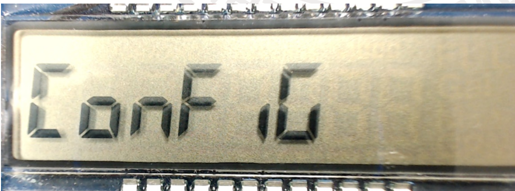
Figure 5. An example of the register display when the optical switch is communicating with the remote capable device.
